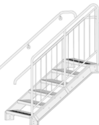
Single flight staircase without landing
