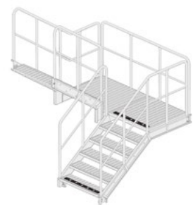
Single flight staircase 180° turning landing
