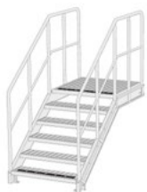
Single flight staircase with landing
