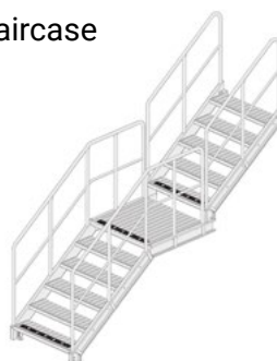
Two-flight staircase with intermediate landing
