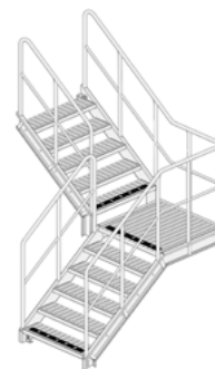
Two-flight staircase 90° turning landing
