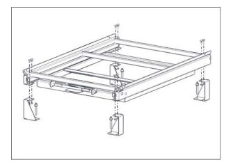
2. The floor model consists of the standard pull-out unit and 4 feet as well as handle. Fasten the four feet to the pullout unit using 2 bolts per foot. Secure the feet to the floor using expander bolts.
