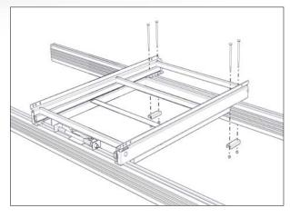
1. Place the pull-out unit across the front and rear support beam(beam model). Secure the rear section of the pullout unit to the rear support beam using enclosed bolts (4 M8) and fixing iron.
