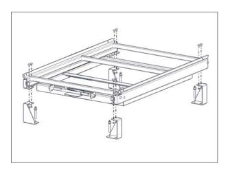
2. The floor model consists of the standard pull-out unit and 4 feet as well as handle. Fasten the four feet to the pullout unit using 2 bolts per foot. Secure the feet to the floor using expander bolts.
