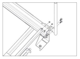
3. Fasten the handle to the pull-out unit using enclosed bolt.
