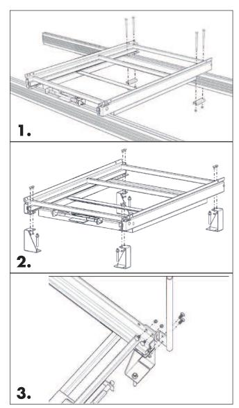
3. Fasten the handle to the pull-out unit using enclosed bolt.
