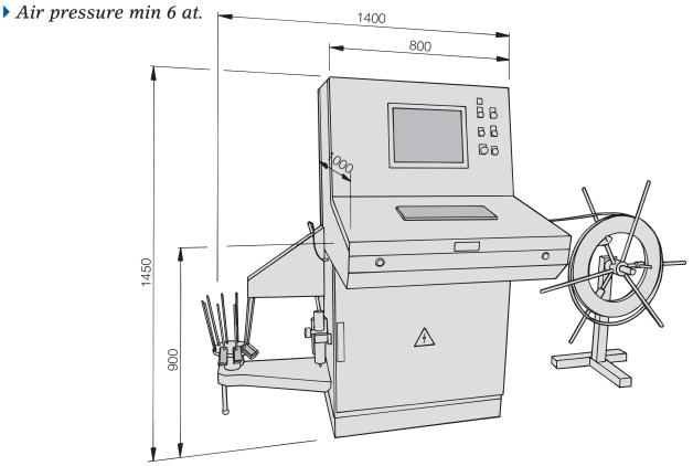
Each tag can be embossed with up to 40 characters. The length of tag varies with the number of characters employed. Holes can be punched at either end or both ends of the tag. Automatic counting of consecutive numbers embossed can be incorporated
