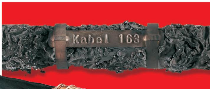
Even after a fire electric cables can be identified.
